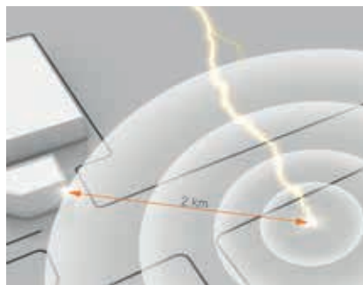
Remote lightning strike Creation of short-term voltage increase in millionths of seconds.
