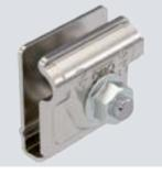
Pre-mounted earthing terminal for the inclusion of PV mounting systems in the equipotential bonding. Suitable for the inclusion of the PV mounting systems in an external lightning protection system. Lightning current-compatible up to 100 kA (10/350)
